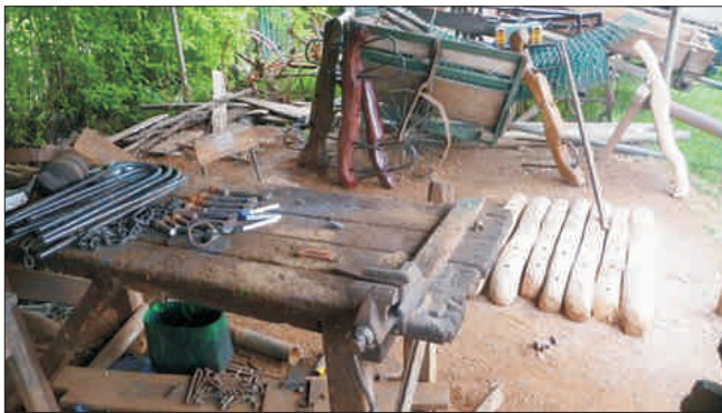
Yokes for ox ploughs and carts are made at the Namalu Centre
